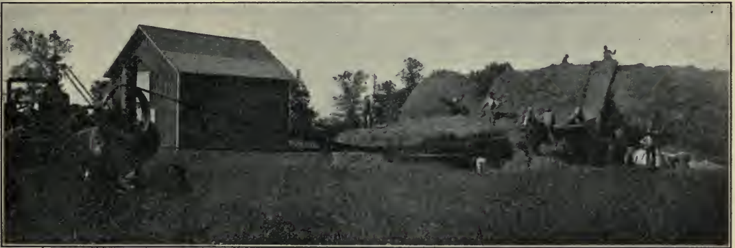
FIG. 241.—A farmer threshing wheat in the harvest season. On the left is an engine which furnishes power to run the threshing machine where the men are standing.
